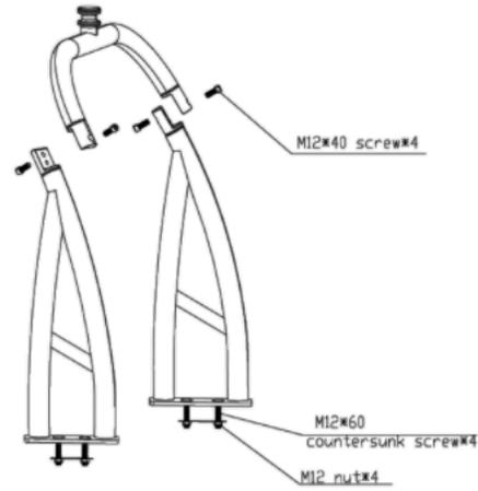
Step1: Assemble the ski tow bar with supplied M12X40 bolts.
