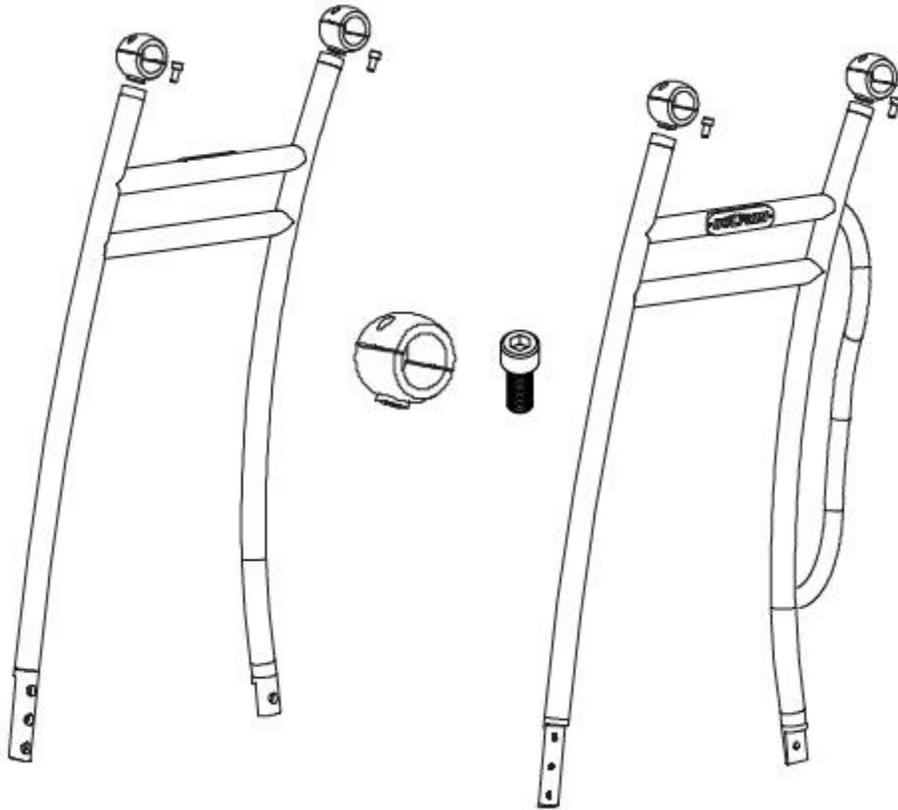
**STEP 5: Assemble the front and center section of the top frame**
