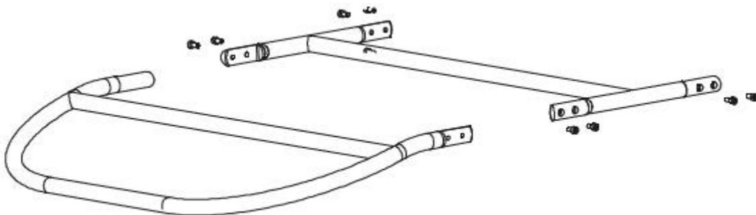
**STEP 6: Attach the Side Supports to the Assemble Top Section**
