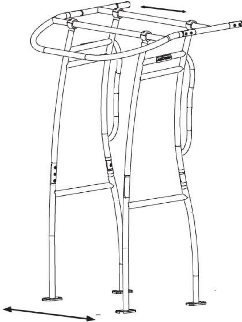
**STEP 7: Attach the T-top to the floor of the boat**
