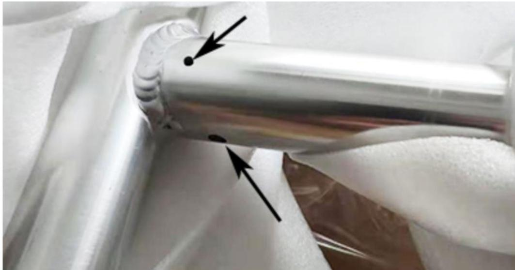
**IMPORTANT:** These small holes should be at the same side of each bar of the top frame. If they are not all on the same side, the legs will not properly attach to the top frame of the t-top. It may appear a half inch too short when attaching the legs. If this is the case, check the holes again.
