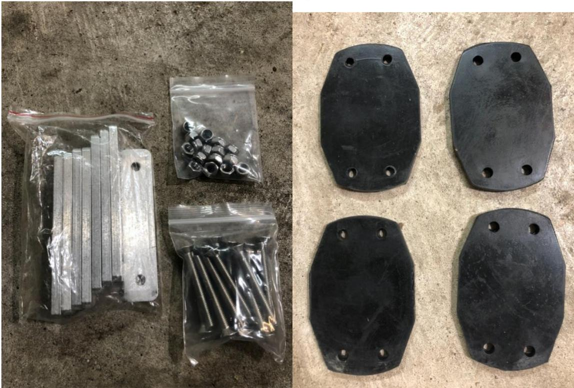
Use the gaskets provided or [3M 5200 Marine Adhesive](#) to seal the t-top feet to the deck. Next, use a phillips head bit to tighten the mounting feet to the deck of the boat. After tightening down all of the screws, recheck them to make sure they are tight. Be careful not to overtighten or strip the screws.
