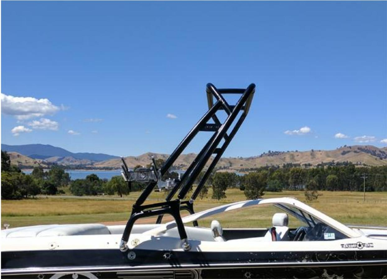
Our Pro Launch Wakeboard Tower uses many common parts with unique design features that make it affordable, adjustable, and easy to install, fast to fold down and erect. Nice designed bracket to hold the tower stay at the position for storage. It is a forward-facing design and there are five main components -- Top Section, Left Leg, Right Leg, side bars and mounting bases.
